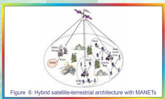
In rural areas, the hybrid architecture can be implemented such that the satellite segment can be utilized to connect the access network nodes like a group of BTS or Node-Bs, in case of PLMNs, scattered in the remote rural areas to the core network node i.e. the BSC in this case. Another scenario could be the traffic aggregated at BSC connected to the MSC using
