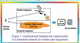
Similar implementation could be there for fixed terminals where a user connected to an ADSL broadband network can be provided high bandwidth consuming services like IPTV or Video on Demand through the satellite segment of the network while other low bandwidth demanding services could be served by the terrestrial (in this case ADSL) network in place. The preferred spectrum is frequency bands allocated to Fixed or Broadcast Satellite Services (FSS or BSS) in Ku or Ka band.
