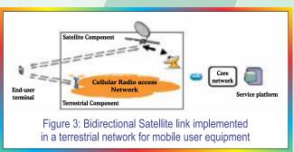
Similar implementation can be done for the fixed terminal equipments where a bidirectional satellite link can be employed in a collaborative manner with the existing terrestrial network, say in this case, an ADSL broadband network. The preferred spectrum is frequency bands allocated to Fixed or Broadcast Satellite Services (FSS or BSS) in Ku or Ka band. Again in this case as well, the pre-deployed infrastructure can be leveraged to add to cost-effectiveness of the system.
