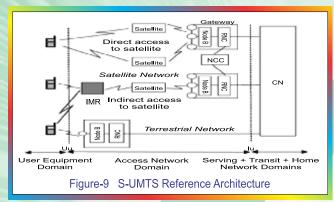
An Intermediate Module Repeater (IMR) is employed in the S-UMTS network which adapts the satellite signals to the MT interfaces and enables full independence from the terminal segment and secondly it improves the satellite coverage in the shadow areas as well as in urban areas where satellite signals inside buildings is highly faded.
