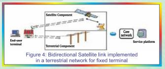
Adding a satellite bidirectional link enables greater flexibility in routing the traffic between both components while at the same time, it ensures a higher resiliency towards potential interruption of service on the terrestrial access link (Typically up to several days or weeks of disruptions). The satellite link
